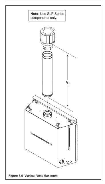
Exhaust restrictors are recommended for these vertically terminated products which have excessive draft. Exhaust restrictors will compensate for high draft, and restore visual flame height. If the vent configuration has a total vertical of 4,6 m - 13,4 m, an exhaust restrictor may be needed. The exhaust restrictor can be located in the appliance manual bag.
